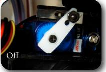
The 'on/off' servo switch for the Nav lights is situated here. When the arm of the servo is pointed aft the lights are 'off', pointed forward they are 'on'.
