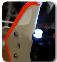
The rear White Nav light is super-gluded (Cyano) to the tail fin and rear tail rotor gearbox. I also heat shrinked the light assembly for easier fitting.
