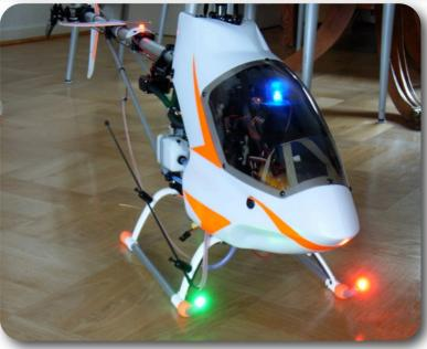
Electrotek R/C Nav lights and Anti Collision light, together with the Blue rapid flashing Gem2000 *All-in-One* warning system LED indicator.
